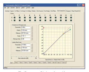
The Compressor/Limiter tab provides a display that enables values to be adjusted with numeric values entered directly, scroll bars to make value adjustments, and dynamic "click and drag" control points on a graphical display.
