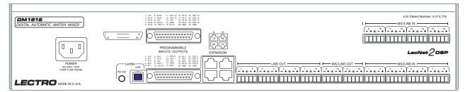
The rear panel of the DM1612 provides all connections for microphones, line inputs, line outputs, external computer control, and EXPANSION ports for "daisy chaining" multiple units or connecting other LecNet2™ devices. Logic I/O ports are also provided for remote control and signaling with external pots, switches and LEDs.
