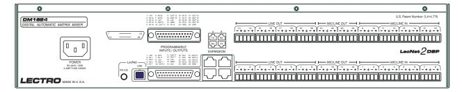
The rear panel of the DM1624 provides all connections for microphones, line inputs, line outputs, external computer control, and EXPANSION ports for "daisy chaining" multiple units or connecting other LecNet2<sup>™</sup> devices. Logic I/O ports are also provided for remote control and signaling with external pots, switches and LEDs.
