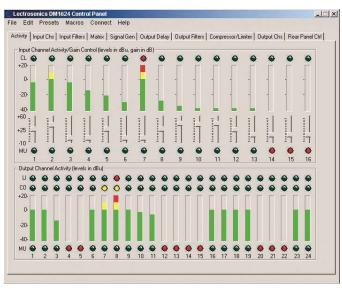
Input and Output signal levels are displayed in a real-time display to monitor the audio activity.
